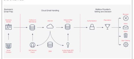
When the ICO sends an email via Sendgrid, the Sendgrid SMTP server processes the email, decides which server to send the message to, and relays the message to that server:
